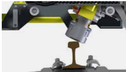
Maximum swivelling range 32° external and 80° internal
